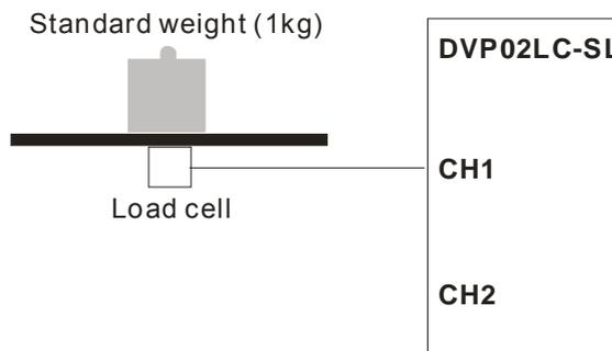
6. Write the weight of the weight (weight base point) into CR#33, as the WPLSoft program below.
