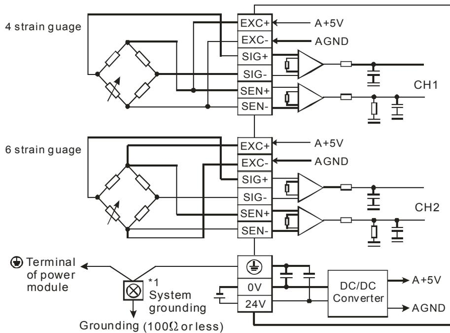
Many load cells connected in parallel connected to a single DVP02LC-SL:
